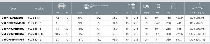
\*\* Free air delivery as per ISO 1217 Annex C, at 14.5 bar at the compressor outlet. ± 3 dB (A) as PNEUROP/CAGI PN-NTC 2.3. Models with air receiver are available on demand
